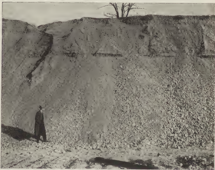
FIG. 9.—The impossibility of obtaining proper and uniform proportion from this average gravel bank is self evident.
